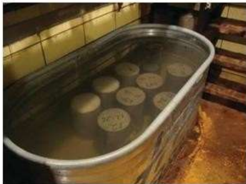
Fig.7:curing concrete specimen
