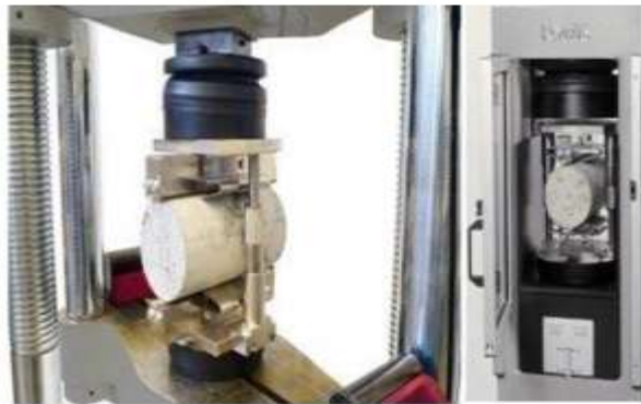
Fig.1: Split cylinder testing machine
